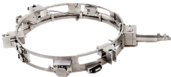
Figure 1 Measurement section with thermocouples to detect transients with higher gradients on piping systems
